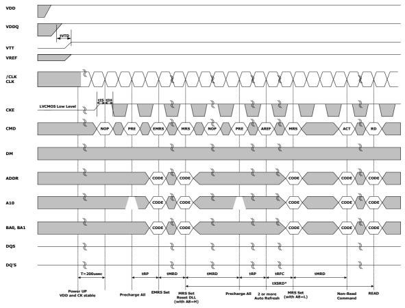
$\boldsymbol{*}$  200 cycle(tXSRD) of CK are required (for DLL locking) before Read Command
